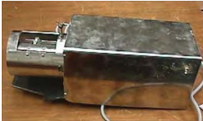
Figure 23 – Mechanical stainless steel oyster grinder
